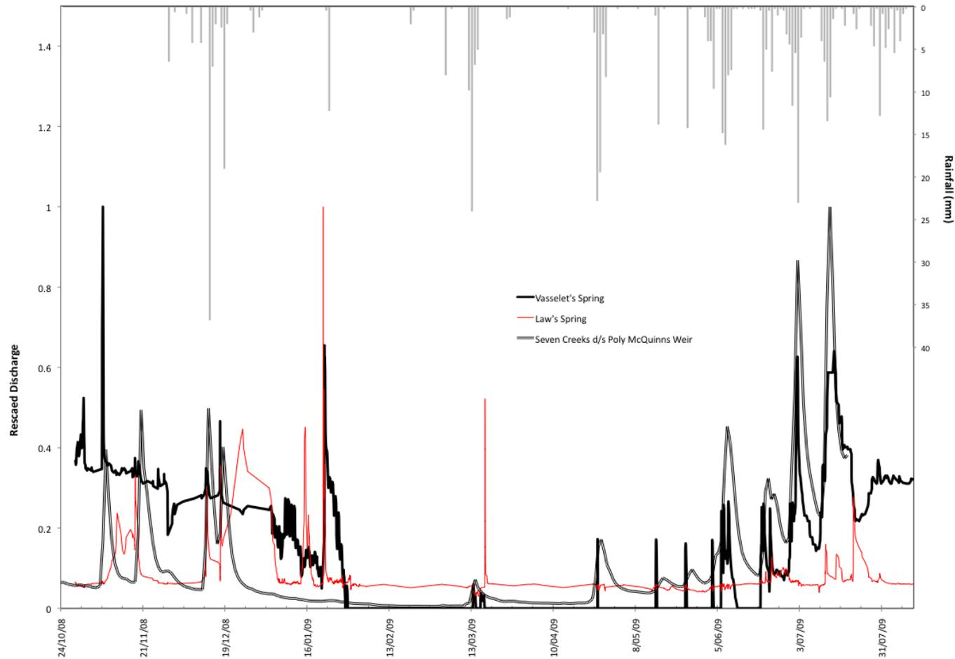
**Figure 5: Discharge at two observation weir downstream of Springs and the Seven Creeks gauge at Polly McQuinn's Weir. Daily rainfall observed at Strathbogie is plotted as a bar graph (with labels on right hand axis). Note that discharge has been re-scaled to allow these to be plotted on the same axis. The value of 1.0 on the y-axis corresponds to 0.025, 0.95 and 120 Ml/d respectively for Vasselet's Spring, Law's Spring and the Seven Creeks gauge.**
