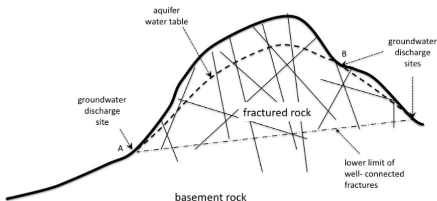
Figure 16: Conceptual model of fractured rock aquifers in the Strathbogie Batholith (modified from Dewandal et al., 2006)
