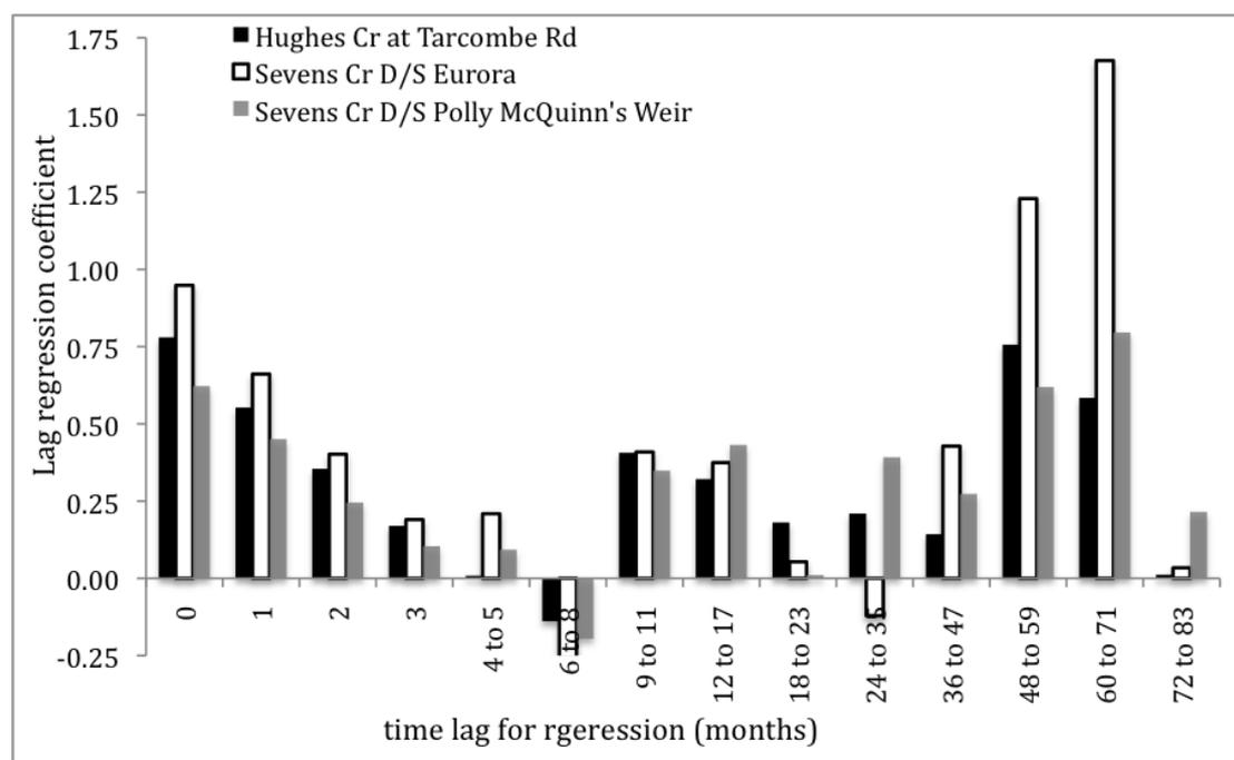
**Figure 6: Coefficients for lag regression model relating ln-transformed monthly rainfall and runoff (n.b. monthly rainfall was averaged over 2 or more months for longer lag periods as indicated by ranges in the x-axis labels)**
