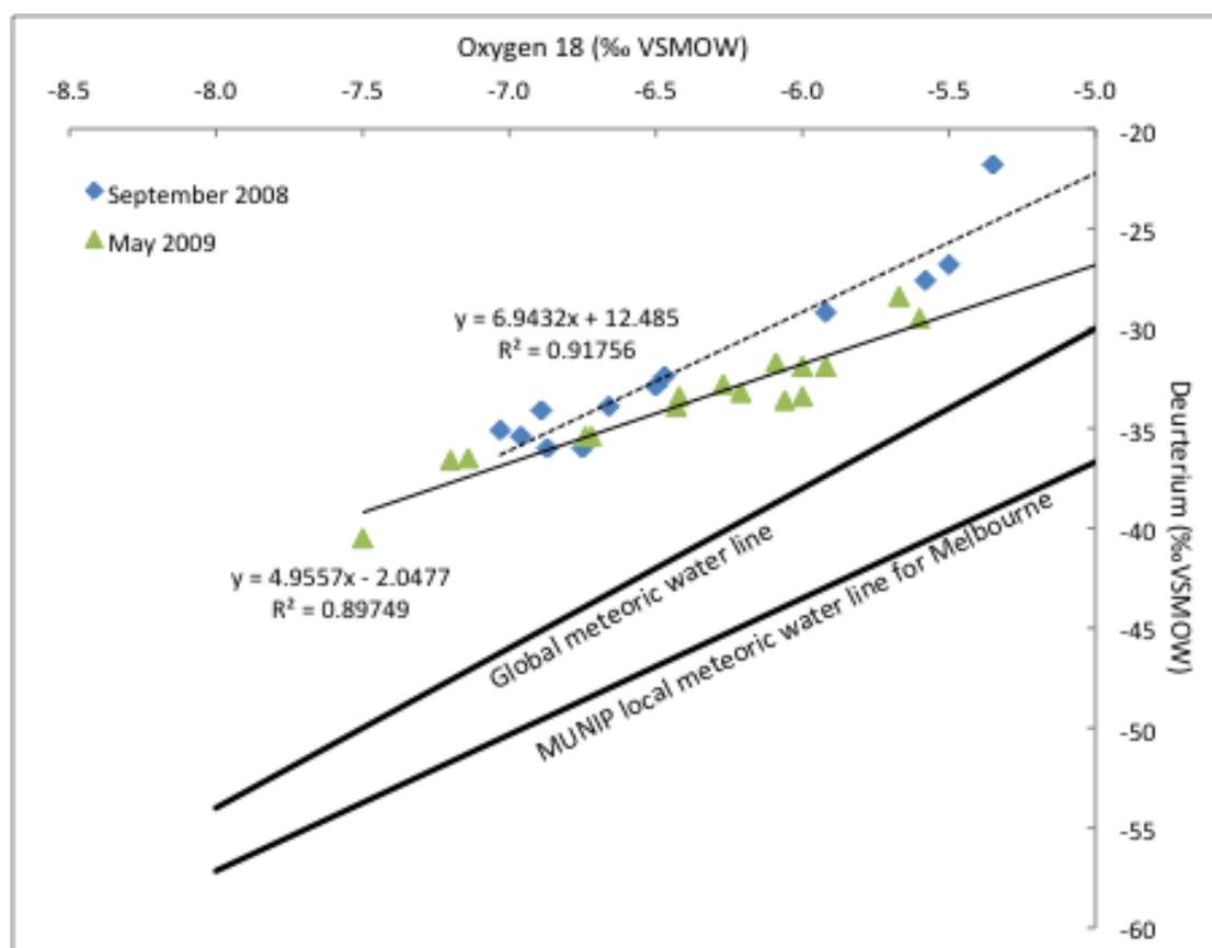
Figure 7: Comparison of Deuterium and oxygen 18 concentration for two sampling times
