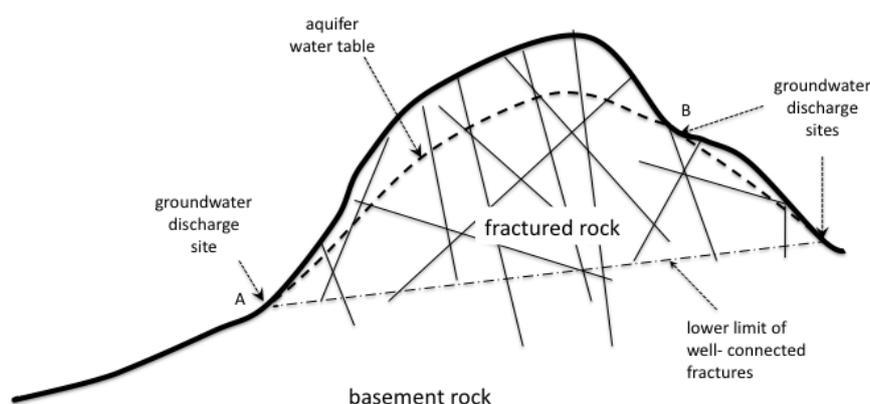
Figure 1: Conceptual model of fractured rock aquifers in the Strathbogie Batholith (adapted from Dewandel et al., 2006)
